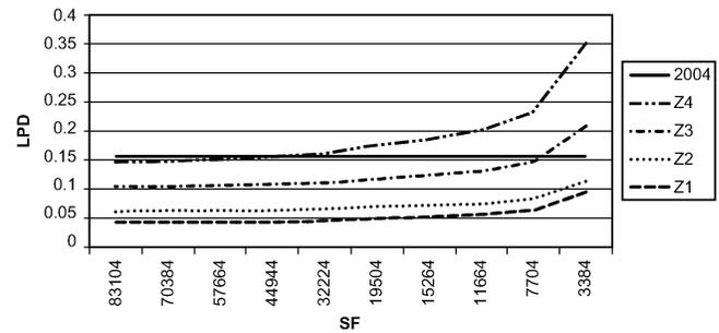
The energy savings from this zone approach is shown in the chart below, with total energy used in each lighting zone for the various square footages. The solid line is the current 2004 standard.
